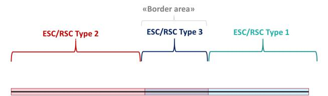
Figure 2 – Ex. 2: ESC/RSC Type border area when the border of all the "ERTMS characteristics" falls within an "area" (option 1)
