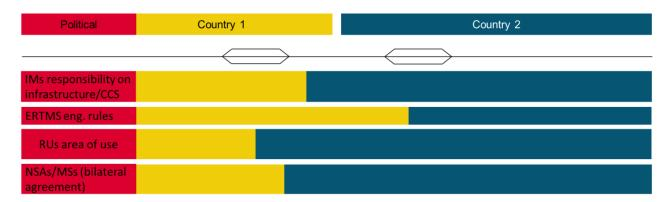
Figure 4 – Example of "ERTMS characteristics" borders not coinciding with the border of NSAs and IMs responsibilities
