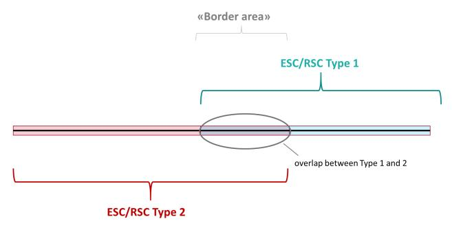
Figure 3 – Ex. 3: of ESC/RSC Type border area when the border of all the "ERTMS characteristics" falls within an "area" (option 2)
