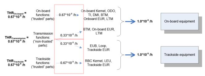
Figure 5 ERTMS/ETCS apportionment between the 3 subsystems
