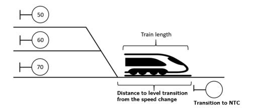
Figure 3: Train length shall be smaller than the distance to the level transition point
