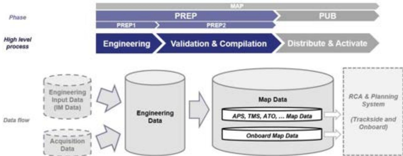
Figure 5 High-level process PREP
