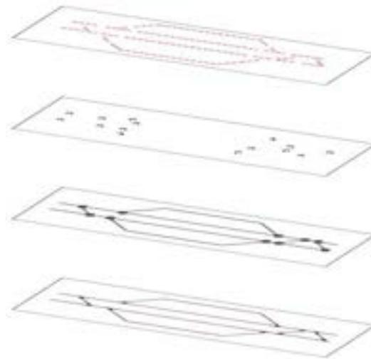
**Figure 6: Layering concept with basic topology, point objects and linear objects**
