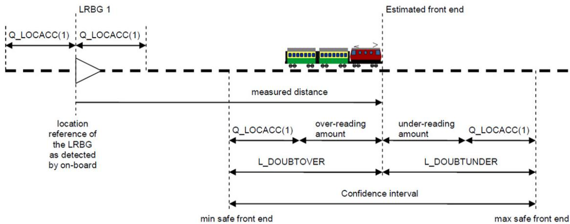
Figure 1: Train Localisation based on ERTMS Subset 026
