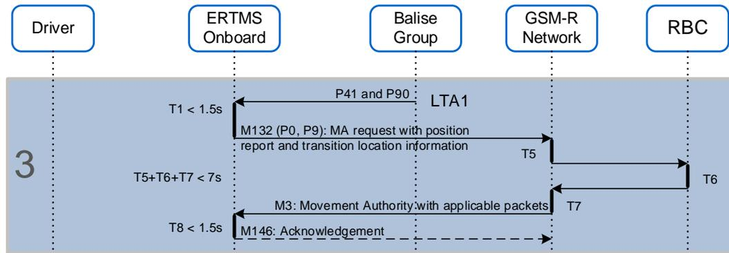
Figure 6: Sequence diagram for solution with MA-request
