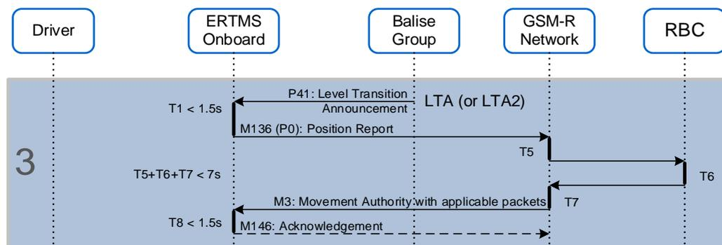
Figure 5: Sequence diagram for solution using position report
