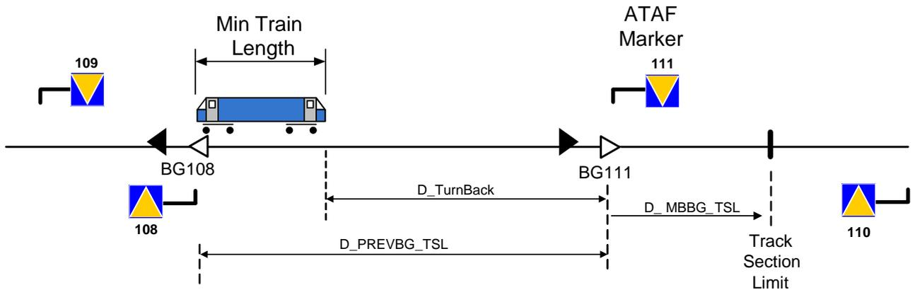
Figure 8: References for the Calculation of the ATAF Distance
