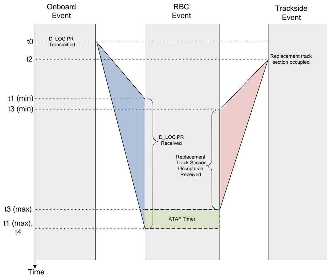
Figure 9 : Calculation of the ATAF Timer Value
