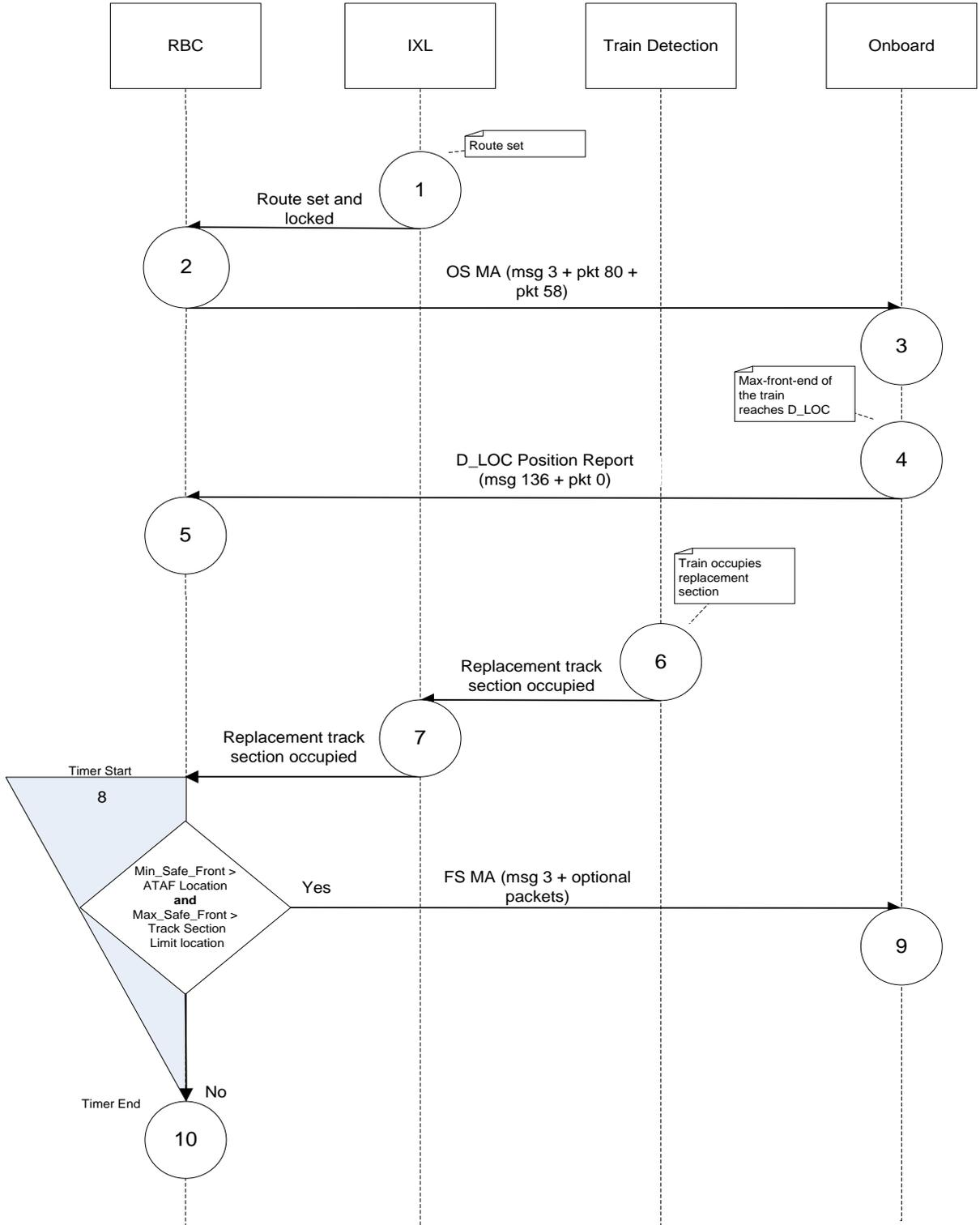
Figure 2: Interaction diagram of ATAF using a position report
