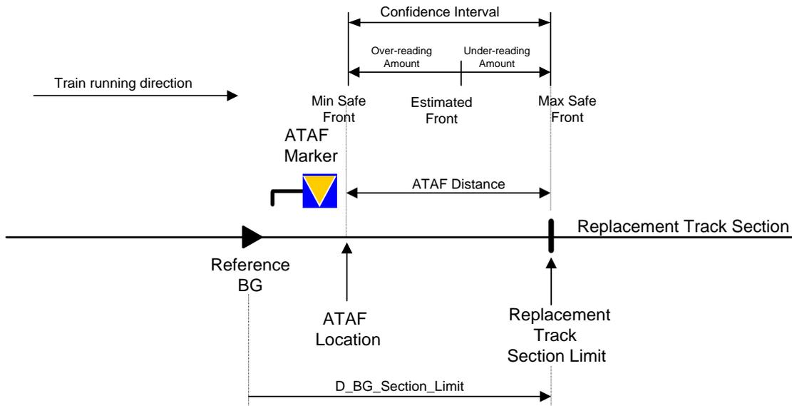
Figure 7: Determining the ATAF Distance
