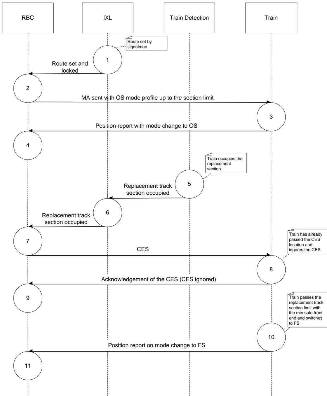
Figure 11: ATAF Interaction diagram using CES method
