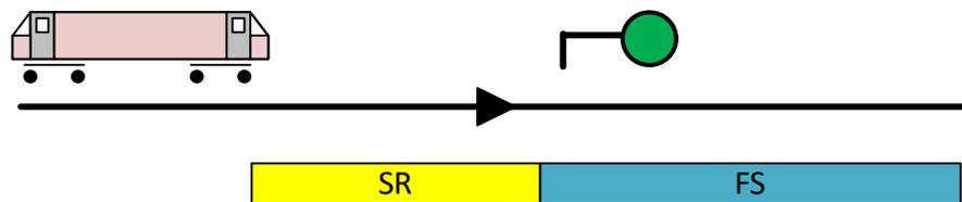
Figure 5 - SoM with optical signal without using the OS mode profile
