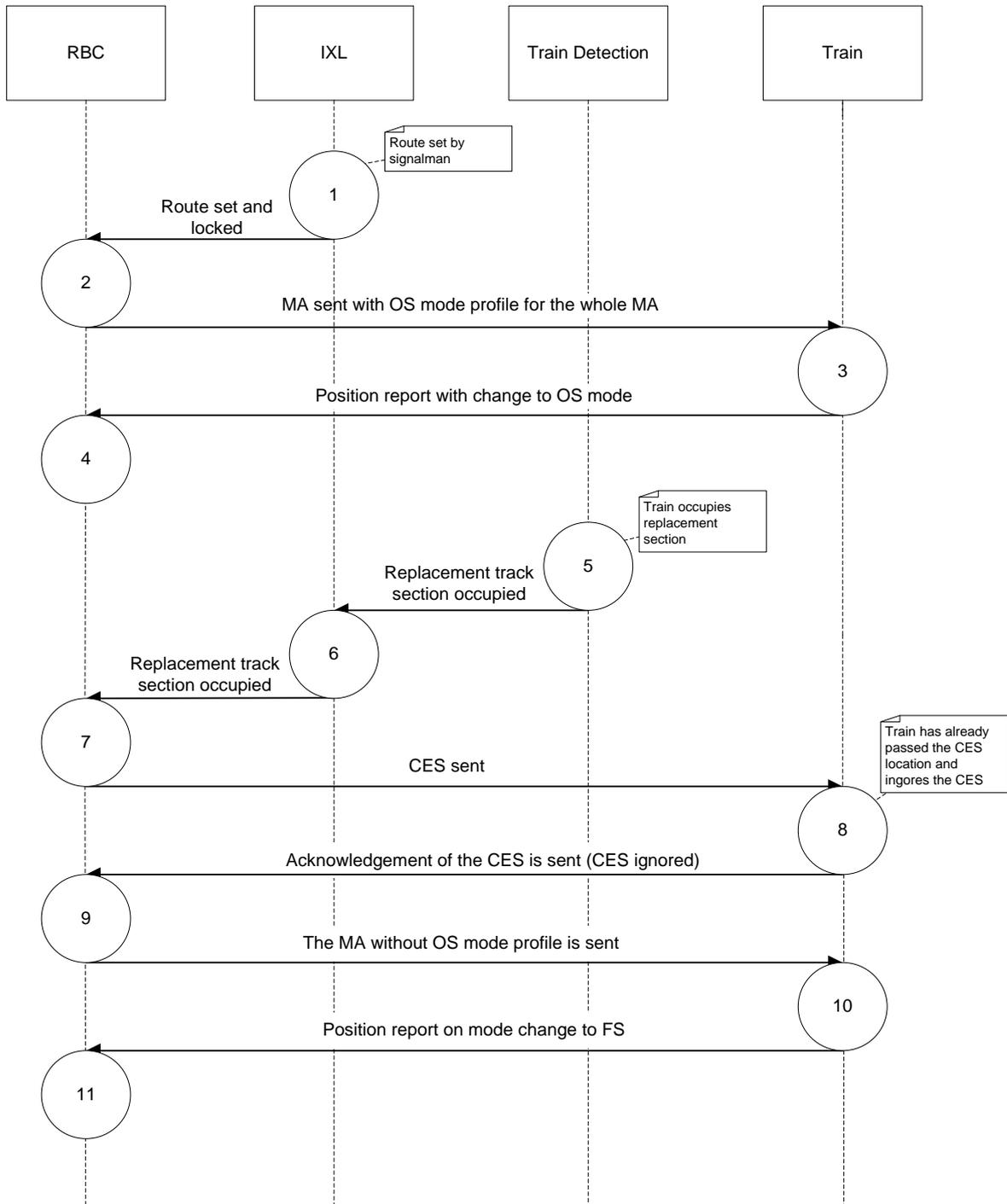
Figure 13: Interaction diagram of pre-check ATAF using CES
